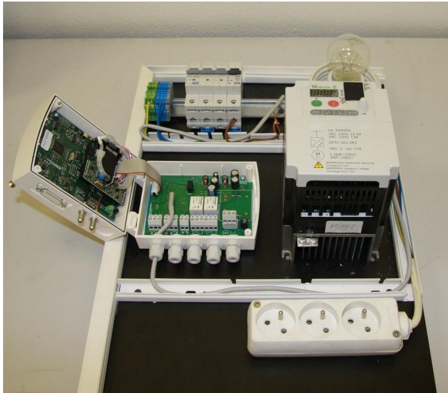
Figure 30 Model of regulation of illumination of the remote experiment
