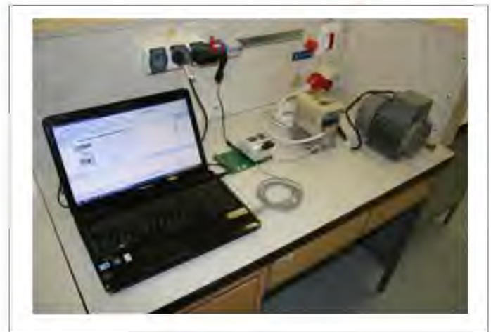
Figure 3. Configuration of the real experiment regarding regulation of the engine revolutions by a frequency changer
