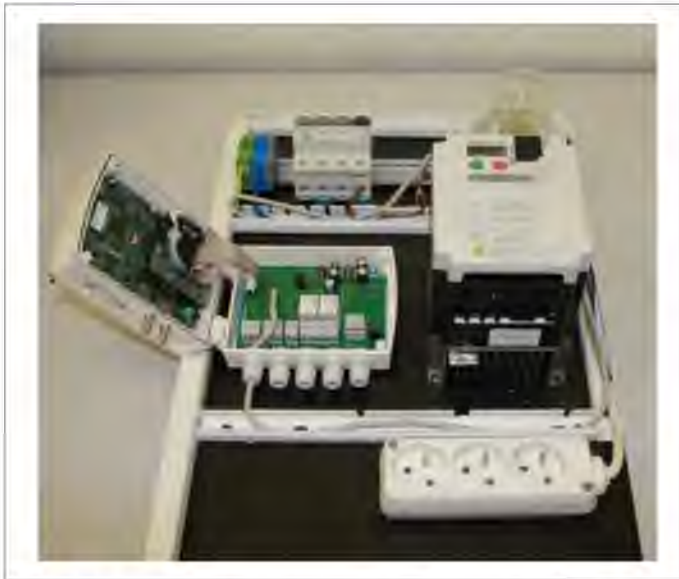
Figure 4. Model of regulation of illumination of the remote experiment in the real laboratory
